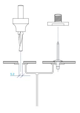
Sometimes panel length is too big and holes with a bigger diameter can not compensate for thermal movement and in such cases oval holes can be cut into the panel. At the same time, one or two round holes should be cut to keep the panel in place. A special cutting drill bit can be used to cut such holes. When a panel is fixed to more than two profiles it is recommended to make the centre of the panel tightly fixed while the sides of the panel are left loose.
