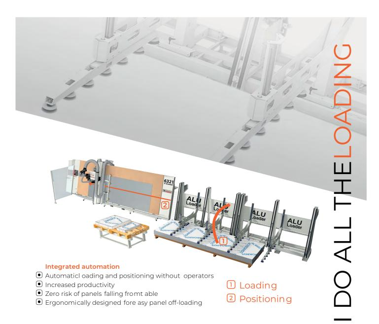
ALU LOADER 42 / 63 / 101 Automatic panel loader for Alu Ranger (Opt.) PATENTED
